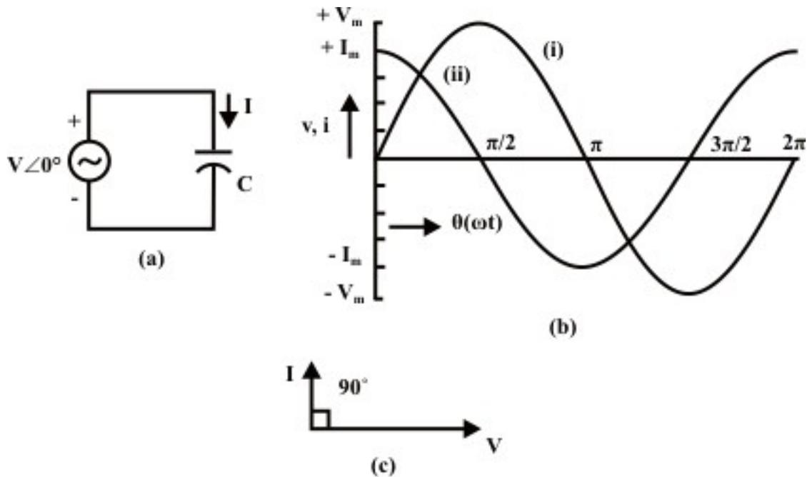
**Fig. 14.3: Circuit with Capacitance (C)**
