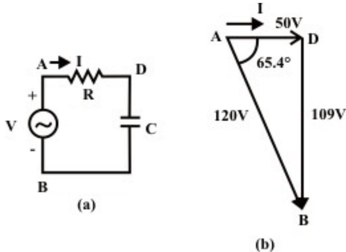
**Fig. 14.7: (a) Circuit diagram
