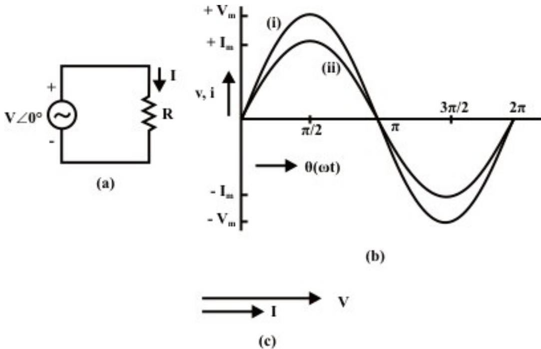
**Fig. 14.1: Circuit with Resistance (R)**
